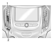
Move the slats (1) to change the direction of the airflow.
