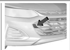
Carefully open the cover in the grille by using the small notch that conceals the tow eye socket.
