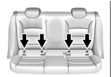
The outboard lower anchors are behind the vertical openings in the seat trim.
