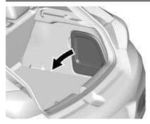
Open and remove the storage compartment door. Store the door under the rear floor storage cover.
