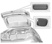
To open the liftgate from the outside, press and on the RKE transmitter to unlock all doors, then use the center touch pad.
