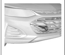
Install the tow eye into the socket and turn it until it is fully tightened. When the tow eye is removed, reinstall the cover with the notch in the original position.
