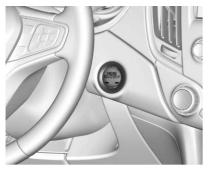
The vehicle may be equipped with an electronic keyless ignition with pushbutton start. The Remote Keyless Entry (RKE) transmitter must be in the vehicle for the system to operate. If the pushbutton start is not working, the vehicle may be near a strong radio antenna signal causing interference to the Keyless Access system. See Remote Keyless Entry (RKE) System Operation (Keyless Access) ⇔ 31 or Remote Keyless Entry (RKE) System Operation (Key Access) ⇔ 38.
