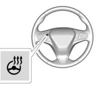
If equipped, press to turn on or off. A light on the button displays when the feature is turned on.
