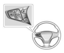
$\mathfrak{F}_{\mathfrak{S}}$ : Press to turn the cruise control system on and off. A white indicator comes on in the instrument cluster when cruise is turned on.
