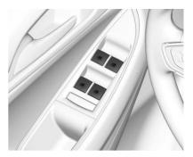
The power windows work when the ignition is on, in ACC/ACCESSORY, or when Retained Accessory Power (RAP) is active. See *Retained Accessory Power (RAP)* ⇔ 180.
