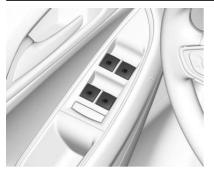
Power windows work when the ignition is on, in ACC/ACCESSORY, or in Retained Accessory Power (RAP). See *Retained Accessory Power (RAP)* ⇔ *180*.
