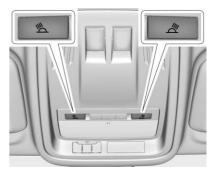
There are front reading lamps on the overhead console.
