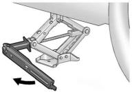
Raise the vehicle by turning the jack handle clockwise. Raise the vehicle far enough off the ground so there is enough room for the road tire to clear the ground. Do not raise the jack any further.
