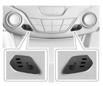
If equipped, the controls are on the center stack. The engine must be running to operate the heated seats.
