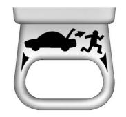
There is a glow-in-the-dark emergency trunk release handle on the trunk lid. The handle will glow following exposure to light. Pull the release handle to open the trunk from the inside.
