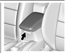
Pull up on the latch to access the storage area.
