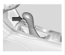
**P**: This position locks the drive wheels. Use P (Park) when starting the engine because the vehicle cannot move easily.
