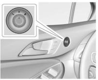
Turn the control knob to L (Left) or R (Right) to choose the driver or passenger mirror. 2. Move the control knob up, down, left, or right to adjust the mirror.
