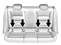
The ISOFIX mounting brackets are located behind the vertical openings in the seat trim and identified with a label on the backrest.
