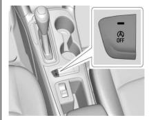
If equipped, the automatic engine Stop/Start feature can be disabled and enabled by pressing the button with the  $(\widehat{A})$  symbol. Auto Stop is enabled each time you start the vehicle.
