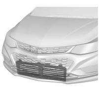
The vehicle may have a shutter system designed to help increase fuel economy. Keep the shutter system clean for proper operation.
