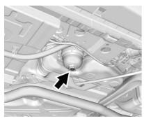
The fuel filter is under the vehicle on the driver side in front of the left rear tire. For replacement of the filter, see *Fuel Filter Replacement* (*Diesel*)  $\Leftrightarrow$  222. Also see Maintenance Schedule ⇔ 325 for recommended draining and replacement intervals.
