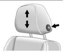
The height of the head restraint can be adjusted. To raise or lower the head restraint, press the button located on the side of the head restraint, and pull up or push the head restraint down, and release the button. Pull and push on the head restraint after the button is released to make sure that it is locked in place.
