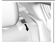
Reach under the seat belt and pull the lever on top of the seatback to unlock the seatback. A tab near the seatback lever moves forward when the seatback is unlocked.
