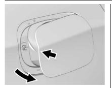
The fuel cap is behind a hinged fuel door on the passenger side of the vehicle. To open the fuel door, push and release the rearward center edge of the door.
