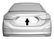
To open the trunk from outside the vehicle, press to twice on the Remote Keyless Entry (RKE) transmitter, or press the touch pad above the license plate after unlocking all doors.
