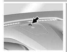
The vehicle has a light sensor on top of the instrument panel. Make sure it is not covered, or the headlamps will be on when they are not needed.
