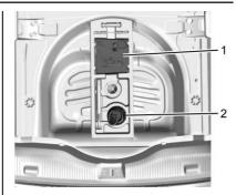
Remove the compressor (1) and the tire sealant canister (2).
