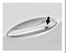
If equipped, press the button on the driver door handle when the RKE transmitter is within 1 m (3 ft) of the driver door handle. When unlocking from the driver door, the first press unlocks that door; press again within five seconds to unlock all passenger doors. See *Remote Keyless Entry (RKE) System Operation (Keyless Access)* ⇔ 31 or *Remote Keyless Entry (RKE) System Operation (Key Access)* ⇔ 38.
