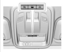
$\stackrel{\text{\tiny $\star$}}{\longrightarrow}$ : Press to turn the lamps off, even when a door is open.
