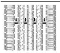
Treadwear indicators are one way to tell when it is time for new tires. Treadwear indicators appear when the tires have only 1.6 mm (1/16 in) or less of tread remaining. See *Tire Inspection*  $\Rightarrow$  285 and *Tire Rotation*  $\Rightarrow$  285.
