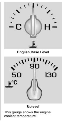
If the pointer moves toward the warning area at the high end of the gauge, the engine is too hot.
