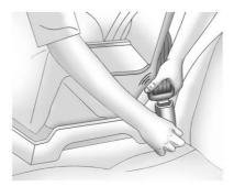
Push the latch plate into the buckle until it clicks. If the latch plate will not go fully into the buckle, check if the correct buckle is being used.
