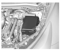
To remove the fuse block cover, squeeze the clips and swing it up.
