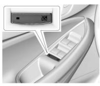
This feature stops the rear door passenger window switches from working.
