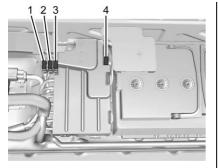
Additional fuses are located near the vehicle battery.
