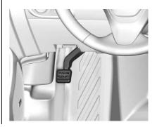
With the brake pedal applied, push the parking brake pedal down. See *Shifting Into Park* ⇔ *180*.
