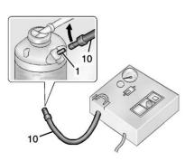
Attach the air only hose (10) to the sealant canister inlet valve (1) by turning it clockwise until tight.
