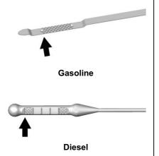
If the oil is below the cross-hatched area at the tip of the dipstick and the engine has been off for at least 15 minutes, add 1 L (1 qt) of the recommended oil and then recheck the level. See "Selecting the Right Engine Oil" later in this section for an explanation of what kind of oil to use. For engine oil crankcase capacity, see *Capacities and Specifications*  $\Rightarrow$  339.
