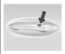
If equipped, the RKE transmitter must be within 1 m (3 ft) of the trunk/liftgate or door being opened. Press the button on the door handle to open. See "Keyless Access Operation" in *Remote Keyless Entry (RKE) System Operation (Keyless Entry (RKE) System Operation (Key Access)* ⇔ 38.
