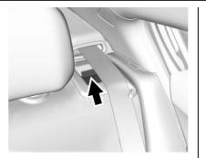
A tab near the seatback lever retracts when the seatback is locked in place.
