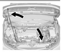
Go to the front of the vehicle and lift the hood and release the hood prop from its retainer, located above the radiator. Securely place the hood prop into the slot on the underside of the hood. To close the hood:
