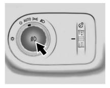
If equipped with front fog lamps, the button is on the exterior lamp control, on the outboard side of the steering wheel.
